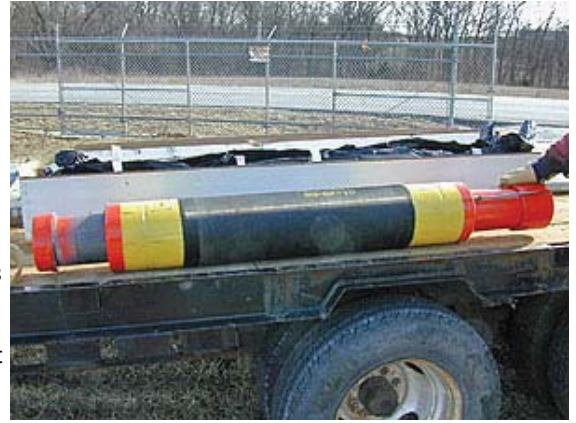
This packer inflates above and below geologic zones to sample water.
